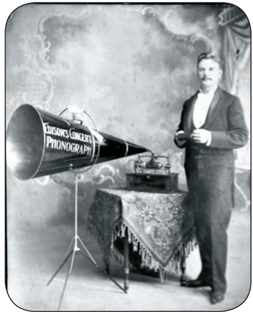
Figure 9. A typical horn around the time Stubbs was travelling. The machine, despite the labelling, is not an Edison but a c.1895 Type K Graphophone. Thanks to George Paul for the photos and info. From Phonographica , by Fabrizio & Paul. Courtesy of the Antique Phonograph Society. Used With Permission.
