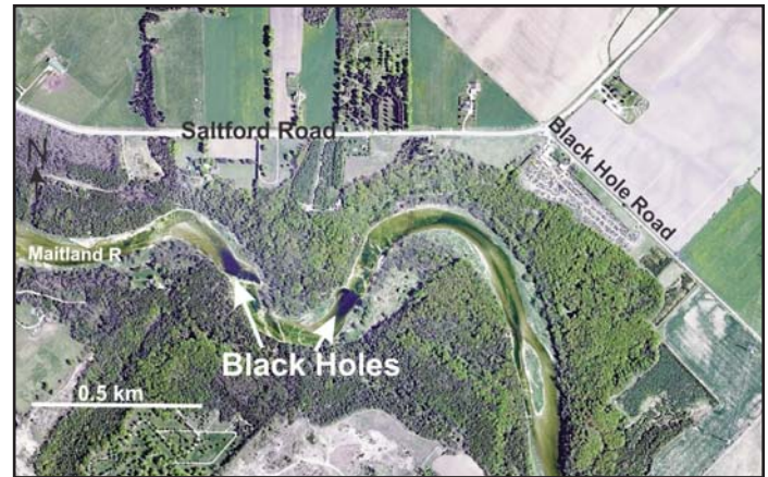
Figure 15. Aerial photograph of the Maitland River west of Goderich showing “black holes” in bed of Maitland River marking location of submerged sinkholes that are over 10 m deep in the Dundee and Lucas formations. The sinkholes provide entry points for infiltration of meteoric water into the bedrock.
