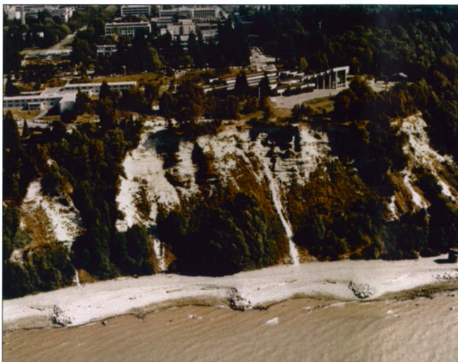
Figure 7 Eroding sea cliff at Point Grey, near Vancouver. The cliff is formed of loose sands and silts. It retreated at rates of up to 60 cm per year before 1982, when coarse gravel was placed at the shore to protect the base of the cliff from wave erosion (University of British Columbia, Campus Planning and Development).
