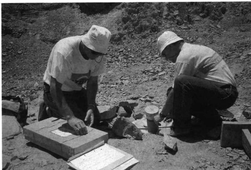
**Figure 2** Workers from the Israeli Geological Survey examine MAZ gold prospect in southern Israel on the occasion of the 18th International Geochemical Exploration Symposium, May, 1997. Large diameter drill hole is capped with a wooden plug (just right of center of photograph), the base of which holds SEM mounts upon which bacteria, living downhole, have accumulated. (Photograph by D. Mossman)
