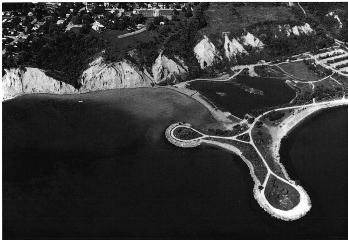
Figure 3 Aerial view of Bluffers Park in September, 1997. Beneath the water level, prominent joints in Pleistocene sediment are expressed as closely spaced black lines perpendicular and parallel to the cliffs to the left of the marina. Joint traces have been widened by waves and accentuated by washed-in cobbles, thus forming dark-coloured lines on the lake floor. The orientation of these joints (Fig. 1B) agrees with the orientation of joints in bedrock (Fig. 1A).
