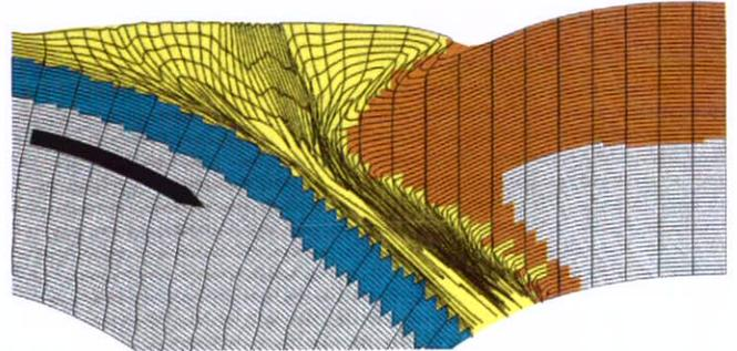
*iii) Mode G: Pro-Wedge, Plug Uplift, Retro-Wedge and Conduit*
