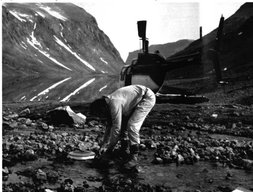
Figure 15 Collecting a heavy mineral concentrate from a small stream bed in northern Labrador for mineralogical and geochemical analysis.
