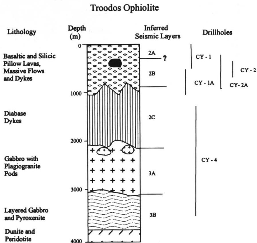
Figure 5 Generalized lithologic section of the Troodos ophiolite showing penetration of boreholes drilled by the International Crustal Research Drilling Group and the inferred correlation with *in situ* oceanic crustal layers. The black feature in the extrusive section is a massive sulphide ore body.
