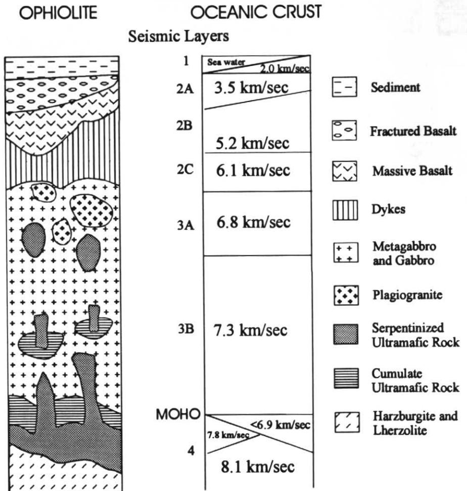
**Figure 3** Generalized composite sections of an ophiolite and *in situ* oceanic crust. Layering in oceanic crust is defined by p-wave velocities which correlate reasonably well with ophiolitic lithologies (e.g., Christensen and Salisbury, 1975). Mantle velocities of 6.9 km·s<sup>-1</sup> represent serpentinized ultramafic rocks and those of 7.8 km·s<sup>-1</sup> correlate with anomalous mantle close to ridge axes.
