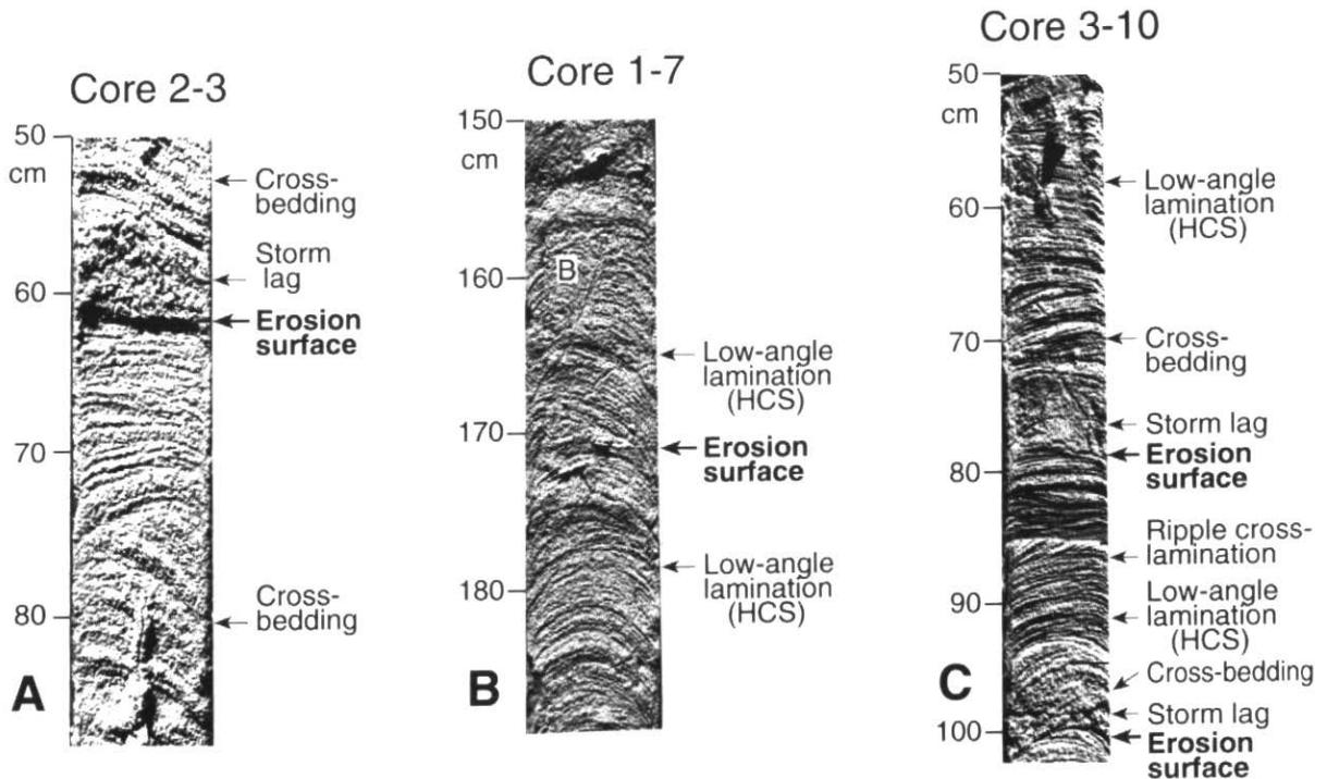
**Figure 8** Core photographs showing: (A) high-angle cross-bedding formed by subaqueous dunes; (B) low-angle lamination (HCS) formed by hummocky megaripples; and (C) event beds containing both high-angle cross-bedding and HCS. Heavy arrows denote erosion surfaces at the base of individual storm-event beds. B=burrow. Scale units in centimetres.
