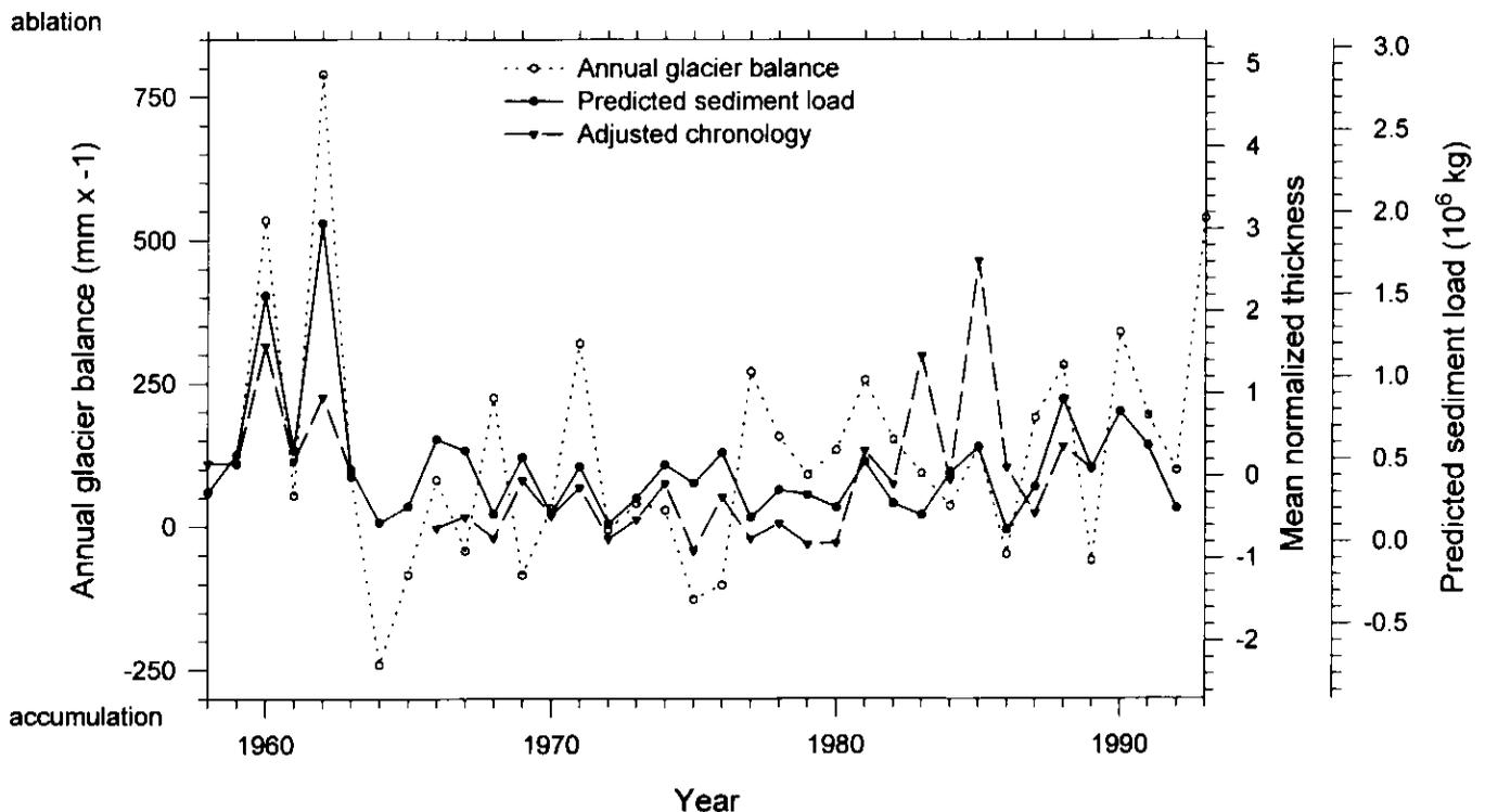
**Figure 4** Predicted annual suspended sediment delivery ( $10^6$  kg) into Lake C2, the adjusted Lake C2 varve chronology (Hardy et al., 1996), and the average annual balance ( $\text{mm} \times -1$ ) for all available Canadian High Arctic glacier data (Koerner, 1995). Sediment flux was predicted by the 600 m sounding temperature at weather station Alert, and can account for 63% of the varve thickness variance. Varve thickness is a mean normalized series ( $n = 8$  cores).
