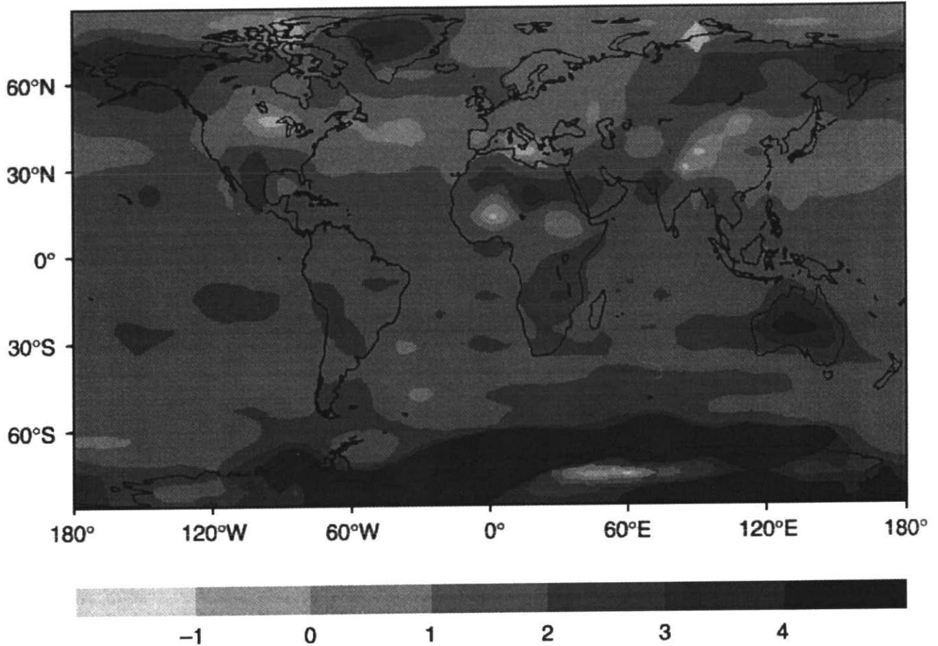
**Figure 1** Change in surface temperature during summer months (June to August) from the period 1880-1889 to 2040-2049, as simulated by a GCM experiment including aerosol effects, and using greenhouse gas forcing from 1880 to 1990, then based on a doubling of equivalent CO<sub>2</sub> after 95 years (Scenario IS92A). Contour interval is 1°C. After Figure 6.10 of Kattenberg *et al.*, 1996.
