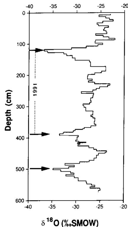
**Figure 5**  $^{18}\text{O}$  record preserved in a snow and firn core from the accumulation area on Bylot Island. The time scale of the core is roughly from July 1992 at the top to summer 1989 at the base. Winter peaks are indicated by arrows.
