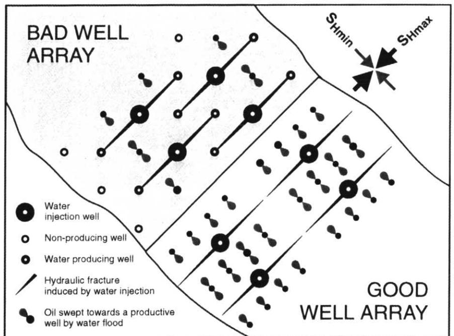
**Figure 8** Production well configurations in an idealized oil field where waterflooding promotes hydraulic fracturing. In the "bad" array, little oil is recovered because induced fractures connect water injection wells with intended production wells. In the "good" array, the induced fractures do not interconnect and distribute the injected water so that it drives oil towards numerous production wells (after Bell and Babcock, 1986).
