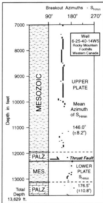
**Figure 4** Breakout orientations measured between 7000 and 13,624 ft in the Amerada Shunda 6-25-40-14W5 well that was drilled in the overthrust foothills along the western margin of the Western Canadian Sedimentary Basin. Note that stress orientations change across the thrust fault at 12,298 ft, suggesting that this is a local surface of geometrical detachment.
