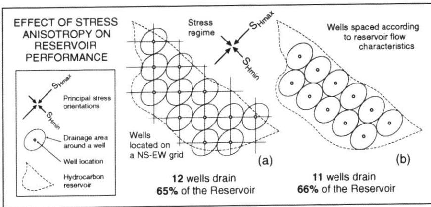
**Figure 11** Schematic representation of how stress-controlled flow anisotropy can affect hydrocarbon recovery from a reservoir that is being produced from vertical wells. In this simplified example, the axis of preferred fluid flow is aligned with  $S_{Hmax}$  (oriented NE-SW), so that the area drained by each well approximates a horizontal ellipse with the long axis oriented NE-SW. The flow preference means that well array (b) will be more productive and cheaper than well array (a).
