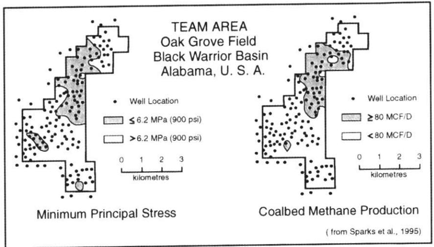
**Figure 17** Relationship between in situ stress and gas production from coal in the Mary Lee Group (depth ca. 700 m) in the Black Warrior Basin, Alabama (Sparks et al., 1995). Note that productivity is greatest where the in situ stress is the lowest.
