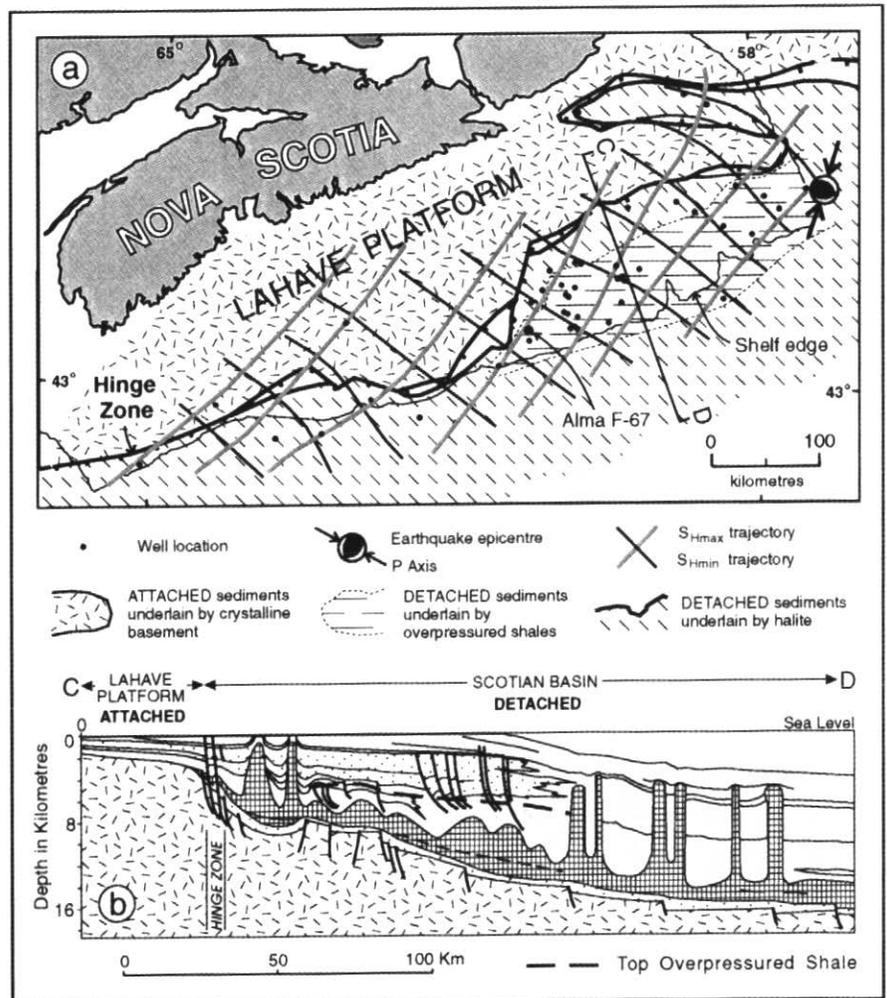
**Figure 5** (a) Stress trajectories derived from breakouts in 54 wells on the Scotian Shelf, offshore eastern Canada (Bell, 1990). The map delineates the inferred attached and detached stress provinces. (b) Cross section through the Scotian Basin showing the postulated attached stress regime above the Lahave Platform and the inferred detached sediments downdip of the Hinge Zone.
