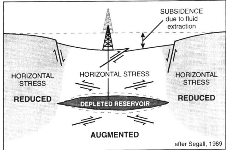
**Figure 23** Schematic cross section showing changes in the stress regime caused fluid withdrawal from an oil field. The net effect is to decrease the horizontal stresses acting around the edge of a field (grey zone) and to increase them above and below it (white zone). As a result, normal faults may develop on the flanks of fields, especially if subsidence is significant, whereas reverse faulting may occur above or below depleted reservoirs.
