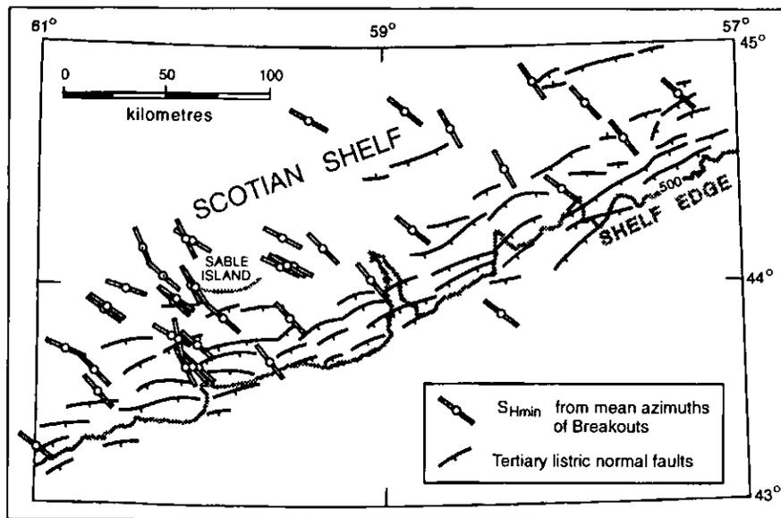
**Figure 26** Map showing the traces of Tertiary listric normal faults compared to the mean breakout azimuths that are diagnostic of today's horizontal principal stresses on the Scotian Shelf. Note that the breakouts are not aligned exactly perpendicular to the fault traces, as would be expected if the faults had evolved in today's stress regime. It would appear that the horizontal stresses have rotated anticlockwise since the faults developed.
