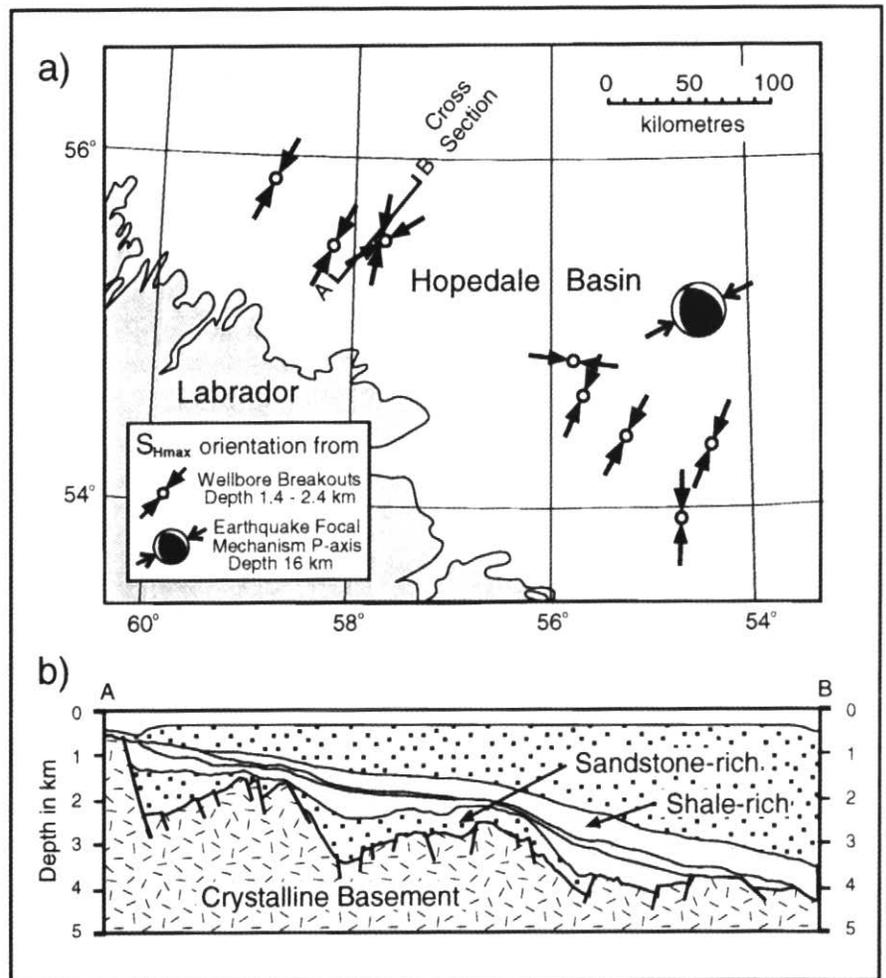
**Figure 2** (a) Map of the southern part of the Labrador Shelf, offshore eastern Canada, where  $S_{Hmax}$  orientations derived from breakouts within Mesozoic and Cenozoic sediments are compatible with the P axis calculated for an earthquake within basement, suggesting an attached stress regime for the sediments. (b) The cross section confirms that there are no potential detachment surfaces between the cover and basement in this part of the Labrador Shelf (after Bell, 1989a).
