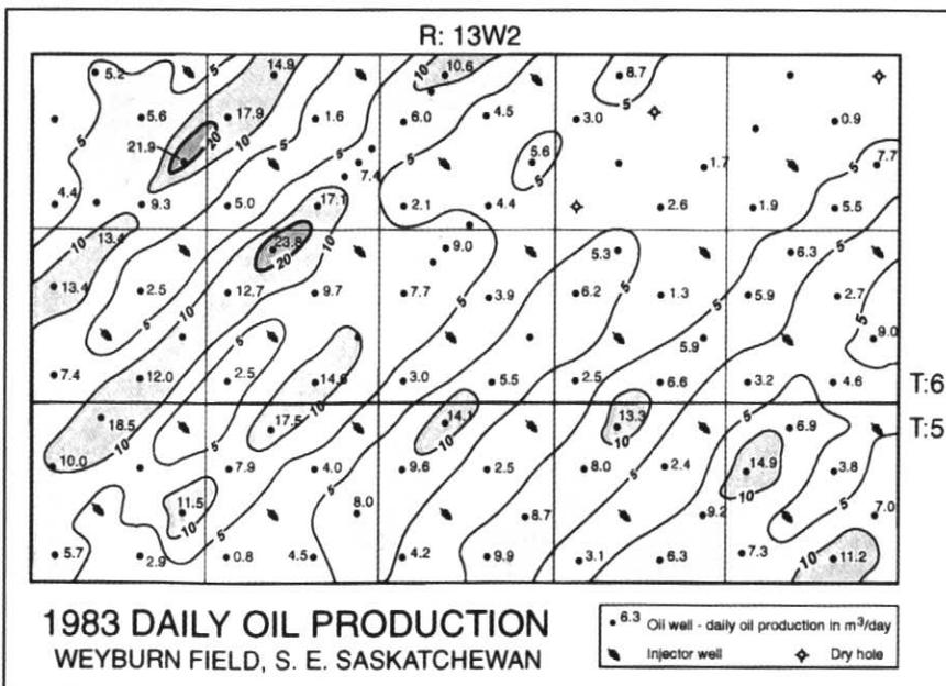
**Figure 10** Daily production rates at Weyburn (Wegelin, 1987) that may reflect stress-induced flow anisotropy in the reservoir.
