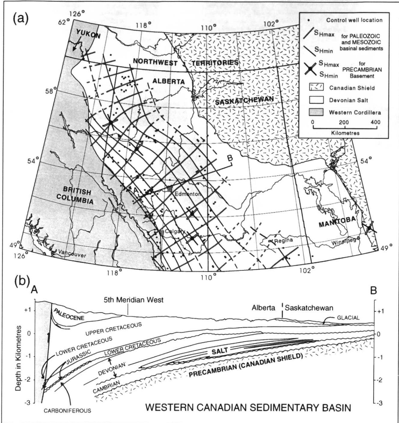
**Figure 3** (a) Stress trajectory map of the Western Canada Sedimentary Basin based largely on mean breakout azimuths from over 200 wells (Bell and McLellan, 1995). Note the similar Precambrian stress axes which imply that the axial and eastern part of basin is attached geomechanically to basement. (b) Simplified dip cross section through the Western Canada Sedimentary Basin. Note the undeformed Devonian salt; it does not appear to have acted as a detachment horizon.
