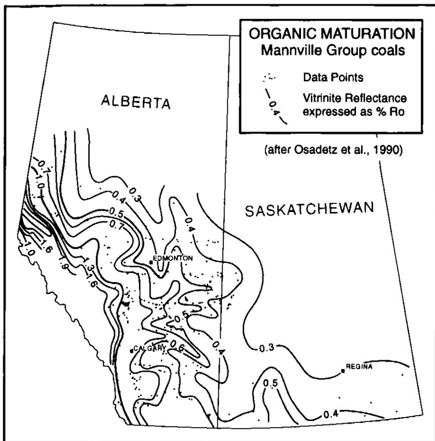
**Figure 25** Mannville Group organic maturation levels (Osadetz et al., 1990) expressed as vitrinite reflectance in oil (% Ro). The map configuration bears no relationship to heat flow patterns and appears to represent the effects of heat transferred by moving fluids, probably along fractures induced by palaeostress regimes!
