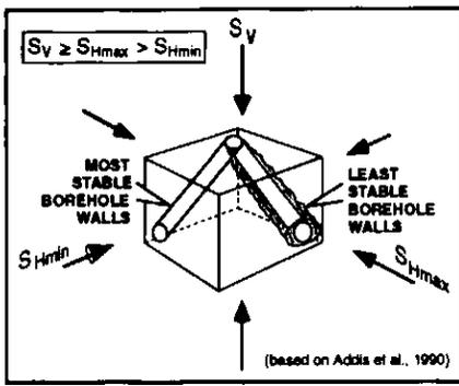
Figure 14 Schematic diagram showing how borehole instability (wall caving) increases when a well is drilled parallel to the plane containing the largest difference in principal stress magnitudes. This situation is similar to what was encountered while developing the Panuke oil field, offshore eastern Canada.
