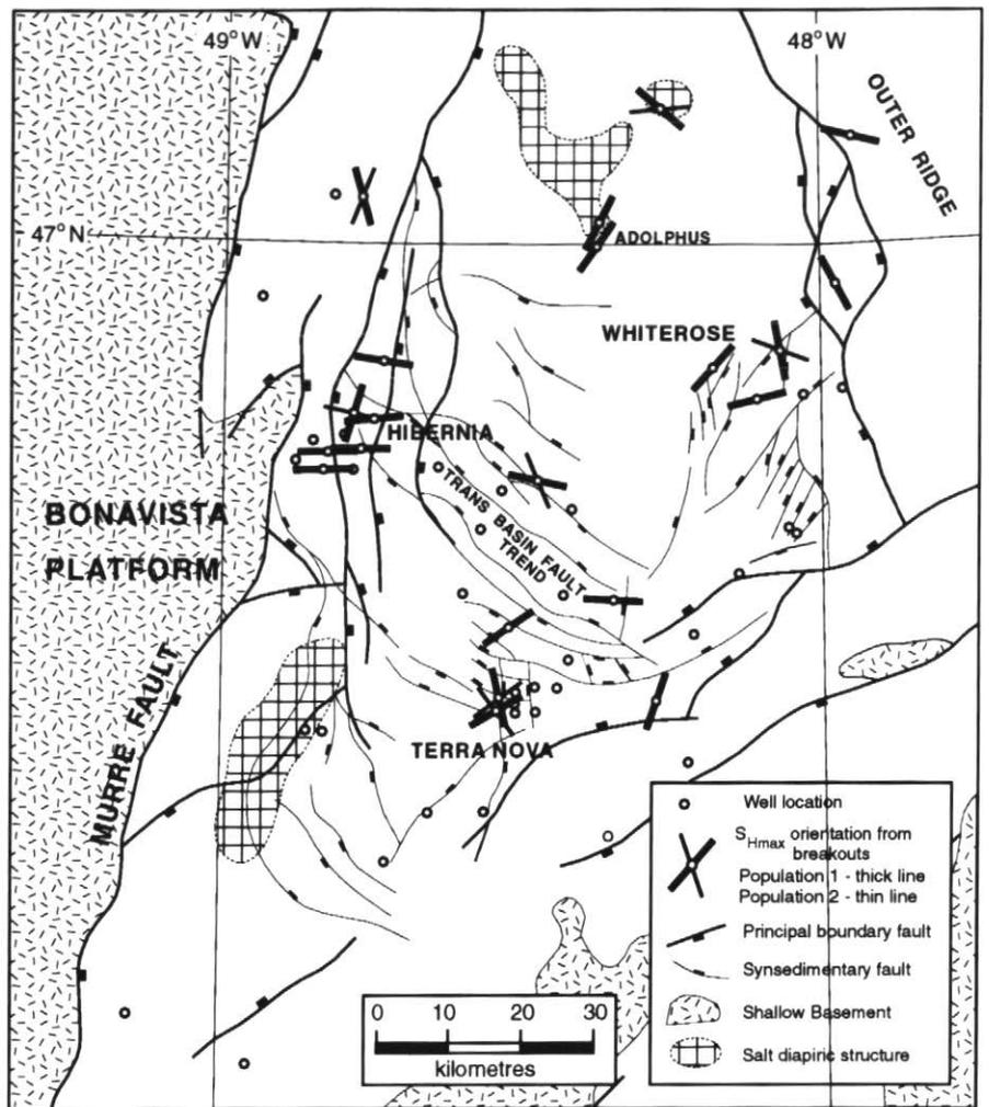
**Figure 7** A preliminary interpretation of horizontal stress orientations in the Jeanne d'Arc Basin of offshore Newfoundland. Most of the breakouts are oriented at high angles to the regional trend (NW-SE) and suggest local horizontal stress deflections related to the elastic properties of fault zones or to geomechanical detachment above overpressured shales and/or halite.
