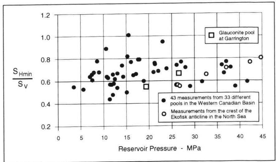
**Figure 18** Plot of reservoir pressures versus  $S_{Hmin}/S_v$  showing how reductions in reservoir fluid pressures lower horizontal stress magnitudes. This is clearly illustrated by measurements made on the crest of the Ekofisk anticline (Teufel et al., 1991). Similar relationships exist in western Canada, as indicated by the data from the Glaucinite pool at Garrington, although the picture appears to be less clearcut when data from 34 pools are plotted on the same graph as shown here.
