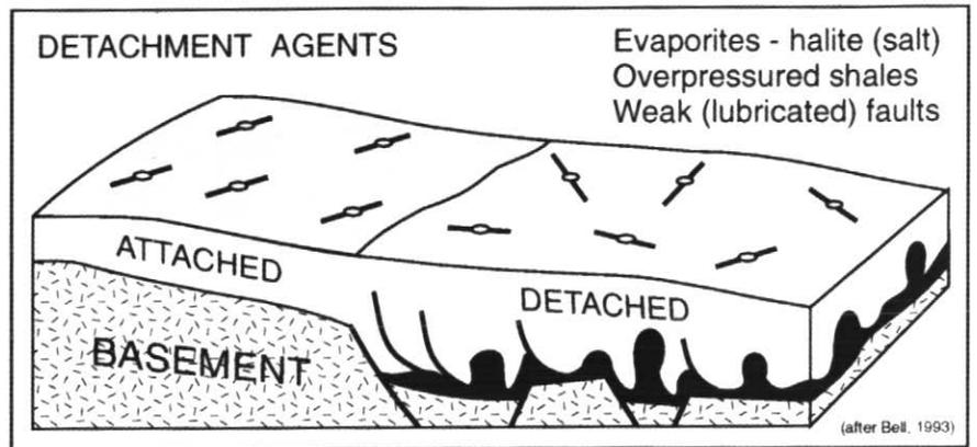
**Figure 1** Schematic diagram of stress regimes that are attached to basement (on left) and detached from basement (on right). Geomechanical detachment can be caused by evaporite layers or overpressured shales (shown in black) and weak sub-horizontal faults (Bell, 1993). Horizontal stress orientations (indicated by the thin bow tie symbols) tend to exhibit more azimuthal variation within detached regimes.
