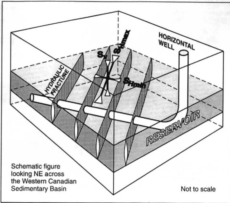
**Figure 9** Hydraulic fractures aligned parallel to  $S_{Hmax}$  induced from a horizontal well drilled parallel to  $S_{Hmin}$  (NW-SE in western Canada). This is the optimum trajectory for a well designed for multiple fracturing.
