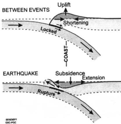
**Figure 7 (Top)** Elastic deformation builds up between great earthquakes if the thrust fault is locked. The seaward edge of the continent is dragged down and a flexural bulge forms farther landward. **(Bottom)** During a great earthquake, there is uplift of the seaward edge and collapse of the flexural bulge. The abrupt uplift generates the tsunami, and the collapse of the bulge causes the subsidence recorded in buried coastal marshes.
