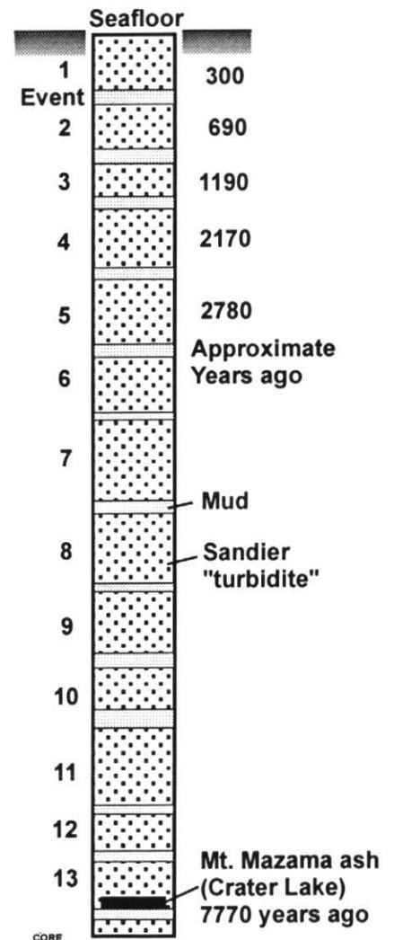
**Figure 6** A 6-m long core sample taken from the deep sea floor shows fine-grained mud layers alternating with sandier layers. The latter are interpreted to have been deposited from submarine landslides triggered by great earthquakes. The mud layers formed by the slow continuous rain of finer sediment settling from the ocean. The volcanic ash at the bottom is dated as 7700 years old (after Adams, 1990).
