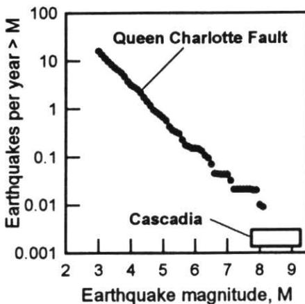
**Figure 2** Earthquakes produced by most fault zones follow the Gutenberg-Richter relation. The average number of earthquakes per year decreases with increasing magnitude. The Queen Charlotte transform (strike-slip) fault zone along the coast to the north of Vancouver Island is typical. The Cascadia thrust fault is unusual in that it produces no small earthquakes, only infrequent very large events.
