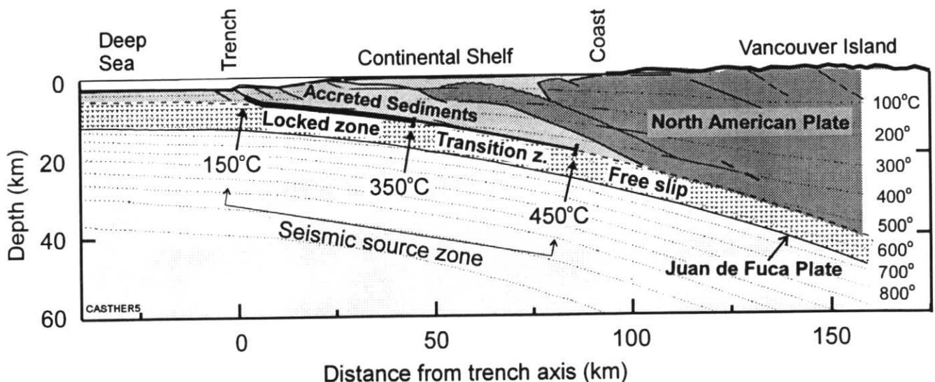
**Figure 12** Cross section through the northern Cascadia margin showing the geological structure and isotherms (lines of constant temperature). The landward limits of the locked and transition zones corresponds to temperatures of approximately 350°C and 450°C, respectively.
