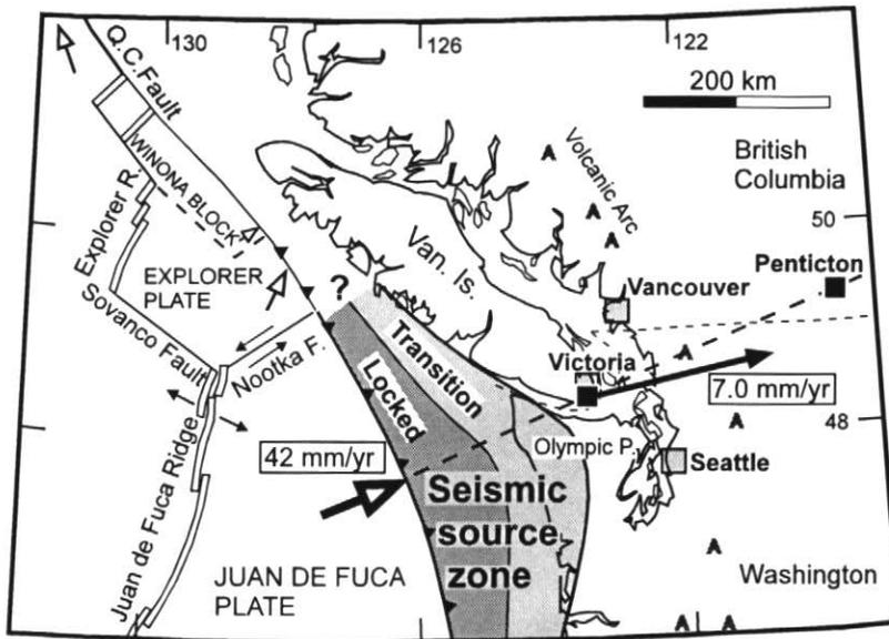
**Figure 8** With the thrust fault locked, the 40 mm·a<sup>-1</sup> convergence of the Juan de Fuca plate is taken up as elastic shortening across the continental margin. GPS measurements show Victoria to be moving landward at a rate of 7 mm·a<sup>-1</sup> with respect to the stable North American continent (Penticton site) (after Dragert and Hyndman, 1995). The remainder of the shortening is across the continental shelf.
