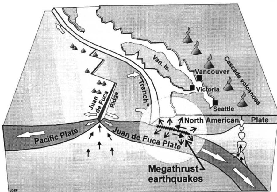
**Figure 1** The Juan de Fuca plate is produced by spreading at the Juan de Fuca ridge several hundred kilometres offshore. It moves landward and beneath the continent at an average rate of  $40 \text{ mm} \cdot \text{a}^{-1}$ . Great earthquakes occur on the Cascadia subduction zone thrust fault contact. Cascade volcanoes such as Mt. Garibaldi and Mt. St. Helens are produced by melting above the downgoing plate where it reaches a depth of approximately 100 km.
