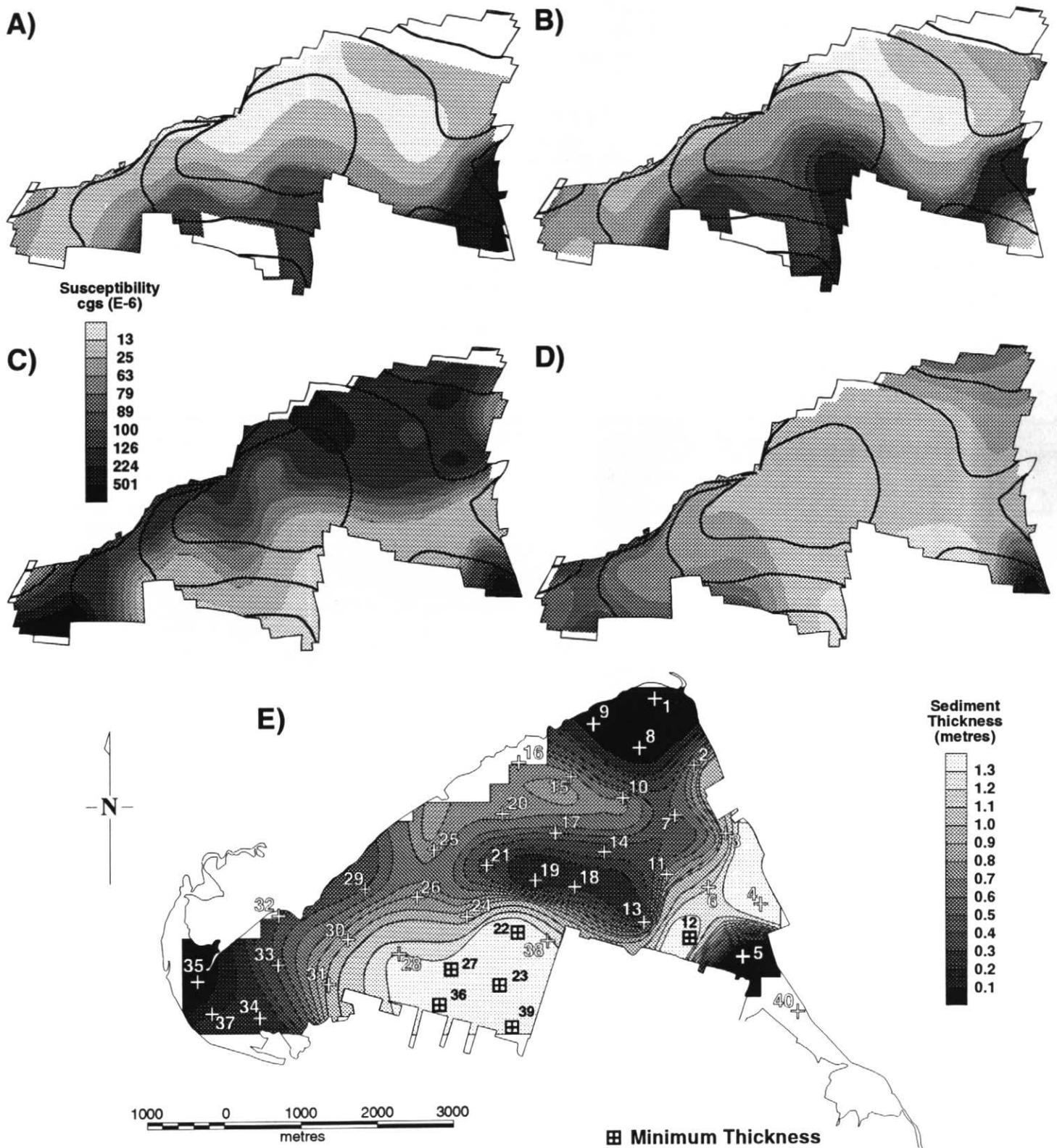
**Figure 4** Contour map of average susceptibility for 10-cm depth slices, draped onto the bathymetry of the harbour. (A) 80-90 cm, (B) 60-70 cm, (C) 40-50 cm, (D) 10-20 cm, bathymetry shown by red lines, depths in metres. Note northward expansion of contamination in successively shallower depth slices. (E) isopach map showing thickness of contaminated sediment in Hamilton Harbour. Thickness and horizontal scale in metres.
