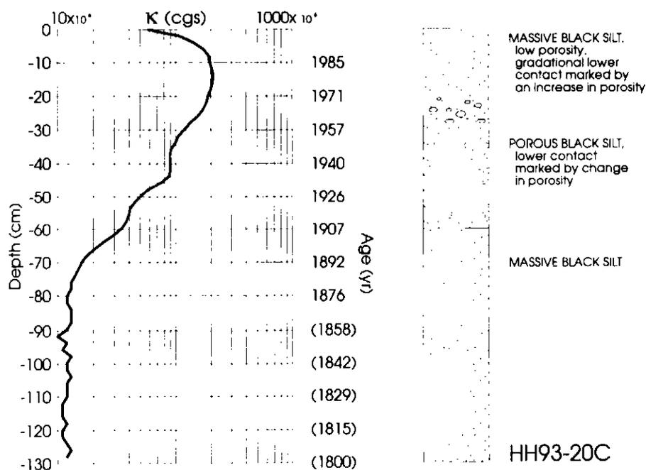
**Figure 2** Typical profile of magnetic susceptibility for Hamilton Harbour core taken at site 20 (Fig. 1). Measurement techniques are described in the text. Ages are  $^{210}\text{Pb}$  ages. Ages in parentheses are extrapolated using calculated sedimentation rates.
