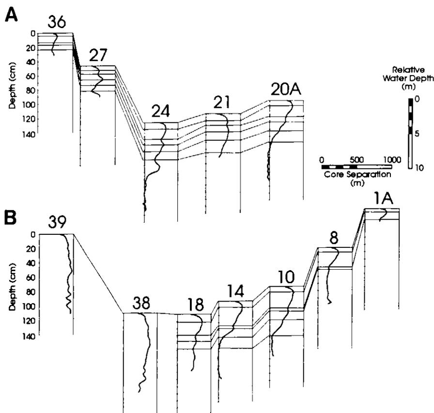
**Figure 3** Correlated cross-sections in Hamilton Harbour. (A) section next to Randle Reef, showing non-disturbed zone. (B) section through Randle Reef showing disturbed sediments along south shore at sites 38 and 39 (Fig. 1). For susceptibility scale, see Figure 2.
