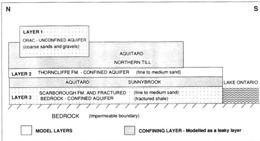
**Figure 11** Design of quasi three-dimensional ground-water flow model based on north-south stratigraphy shown in Figure 5 (from Smart, 1994). The figure identifies model layers only and does not attempt to portray thickness or extent (see Fig. 4).
