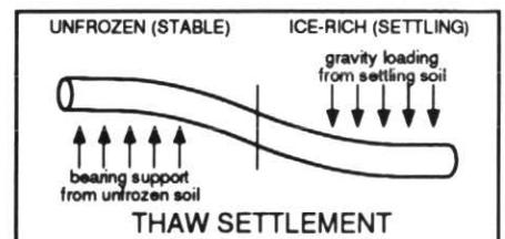
**Figure 11** Conceptual illustration of the freezing and thawing effects of a pipeline crossing from unfrozen to frozen terrain, or vice-versa, in the discontinuous permafrost zone in Canada (from Nixon, 1990).
