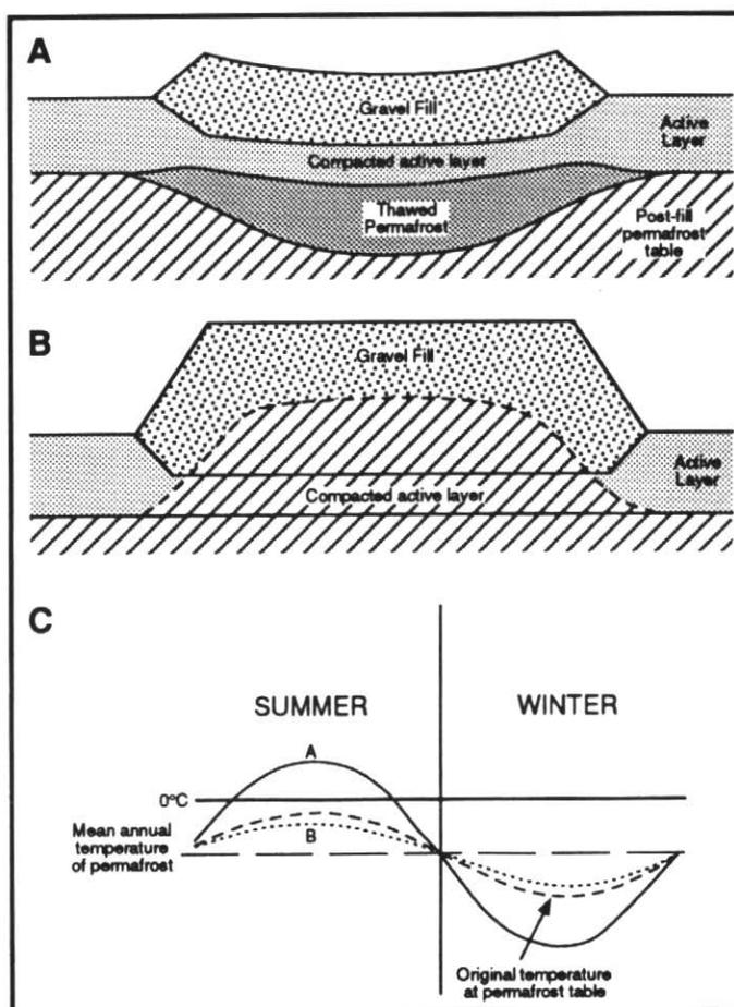
**Figure 4** Diagram illustrating the effects of a gravel fill upon the thermal regime and thickness of the active layer. (A) Too little fill; (B) Too much fill; (C) Effects of cases (A) and (B) upon the thermal regime; too little fill increases the amplitude of seasonal temperature fluctuation at the permafrost table and promotes the development of subsidence (thermokarst; from Ferrians *et al.*, 1969).
