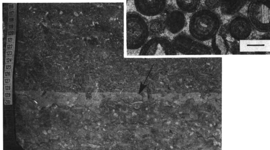
Figure 6 An irregular submarine hardground (between 129 and 128 cm. on the tape) developed in Lower Cambrian ooid limestones of the Forteau Formation, western Newfoundland.
