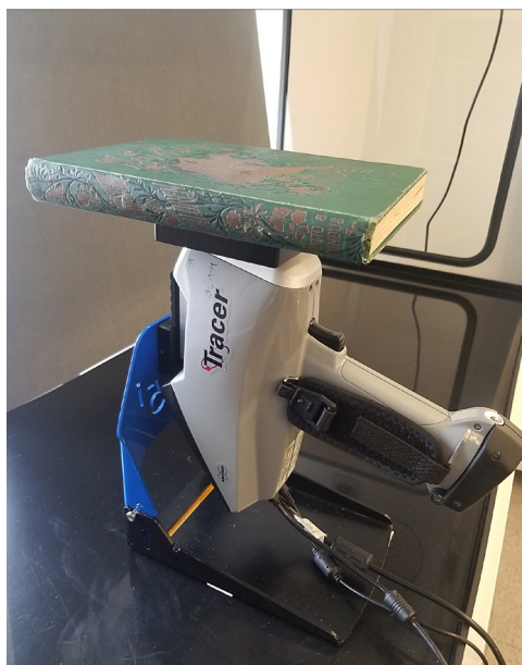
FIGURE 3 Photograph depicting the pXRF setup. Books were placed on top of the sample stage accessory for testing. Photo credit: Robin Canham.
