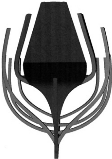
Figure 14. Transom of Indeavour shown from directly astern showing the characteristic “lute” shape transom, as drawn by author.
