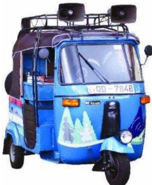
Figure 1. The e-tuktuk, an autorickshaw that serves as a mobile radio station and multimedia centre. Source: Google Images
