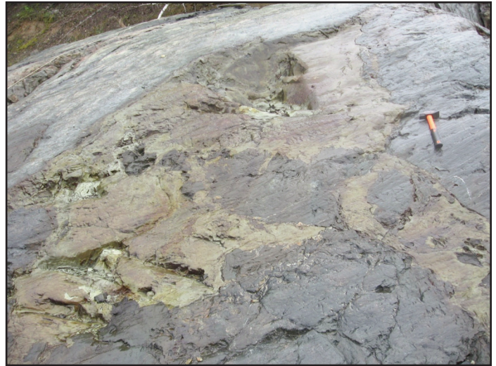
Sharp-walled massive chalcopyrite veins at the Podolsky North Zone in the Whistle embayment of the Sudbury Structure. Photograph courtesy of Bruno Lafrance.
