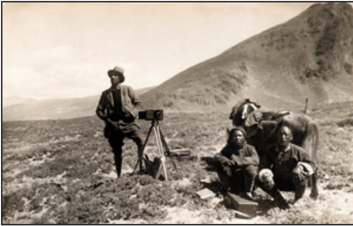
Figure 5. E.O. Wheeler and two of his three Tibetan assistants: Gorang, Lagay and Ang Pasang. Using a Canadian-designed photo-topographical survey camera with 12 x 17 cm plates, Wheeler took 240 single images and panoramas of the northern, western and eastern approaches to Everest, from which the first accurate topographical map of the area was constructed (Fig. 6). The technique required clear and relatively calm conditions, seldom encountered at elevations above 5000 m (wrt sea level) where the team worked for long periods. Photograph in 1921 by Sandy Wolston courtesy of the Royal Geographical Society.
