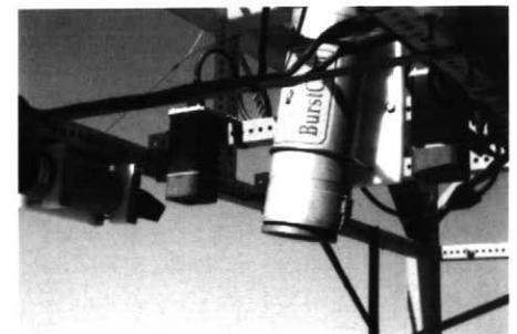
**Figure 6** Photograph showing the Mesotech 2.2-MHz acoustic backscatter sensors (rectangular cylinders) and the 675-kHz Imagenex Sector Scanning Profiler (far-left cylinder with a flat head) mounted on the GSC-instrumented platform RALPH.
