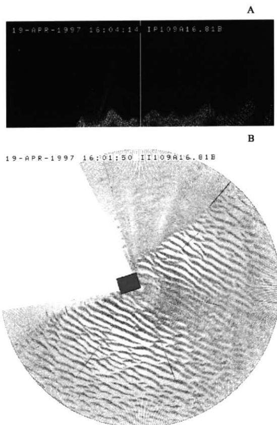
**Figure 9** Example seabed images recorded by the Imagenex Sector Scanning sonars. (A) the vertical profile of the seabed scanned by the sector scanning profiler. The length of the image is about 5 m and the vertical height is about 130 cm. The white band indicates the bedforms with a maximum height of 18 cm. (B) the 270° image recorded by a sector scanning imager. The image has a 40 m diameter and displays large wave ripples of 1 m average wavelength.
