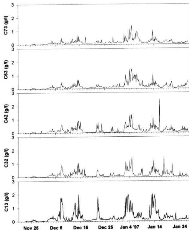
**Figure 5** Profiles of mean suspended sediment concentration measured by the OBS array on an instrumented tripod (courtesy of D.A. Hepworth, C.T. Friedrichs, and L.D. Wright of Virginia Institute of Marine Science).
