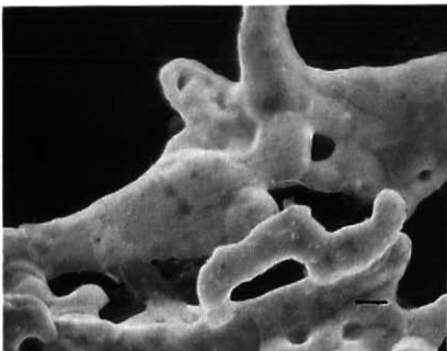
Figure 6 Characteristic microfossil-like filamentous structure of gold extracted from oxidized carbonaceous matter (kerogen) from the Carbon Reef Leader, Witwatersrand. Scale bar (lower right) = 2µm. (Photograph courtesy of Dr. D.K. Hallbauer, University of Pretoria)
