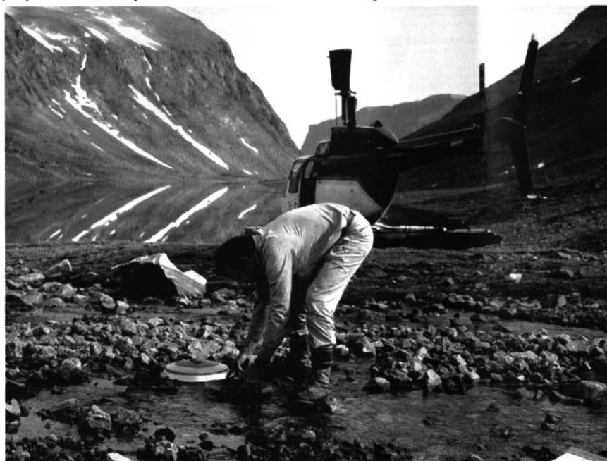
Figure 15 Collecting a heavy mineral concentrate from a small stream bed in northern Labrador for mineralogical and geochemical analysis.
