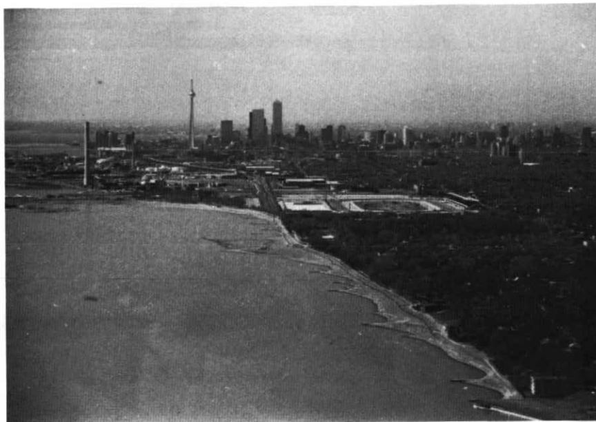
Figure 8 View looking west of the Eastern Beaches (Fig. 2) toward the downtown core showing groynes and resulting entrapment of littoral sediment transported by the long shore drift system
