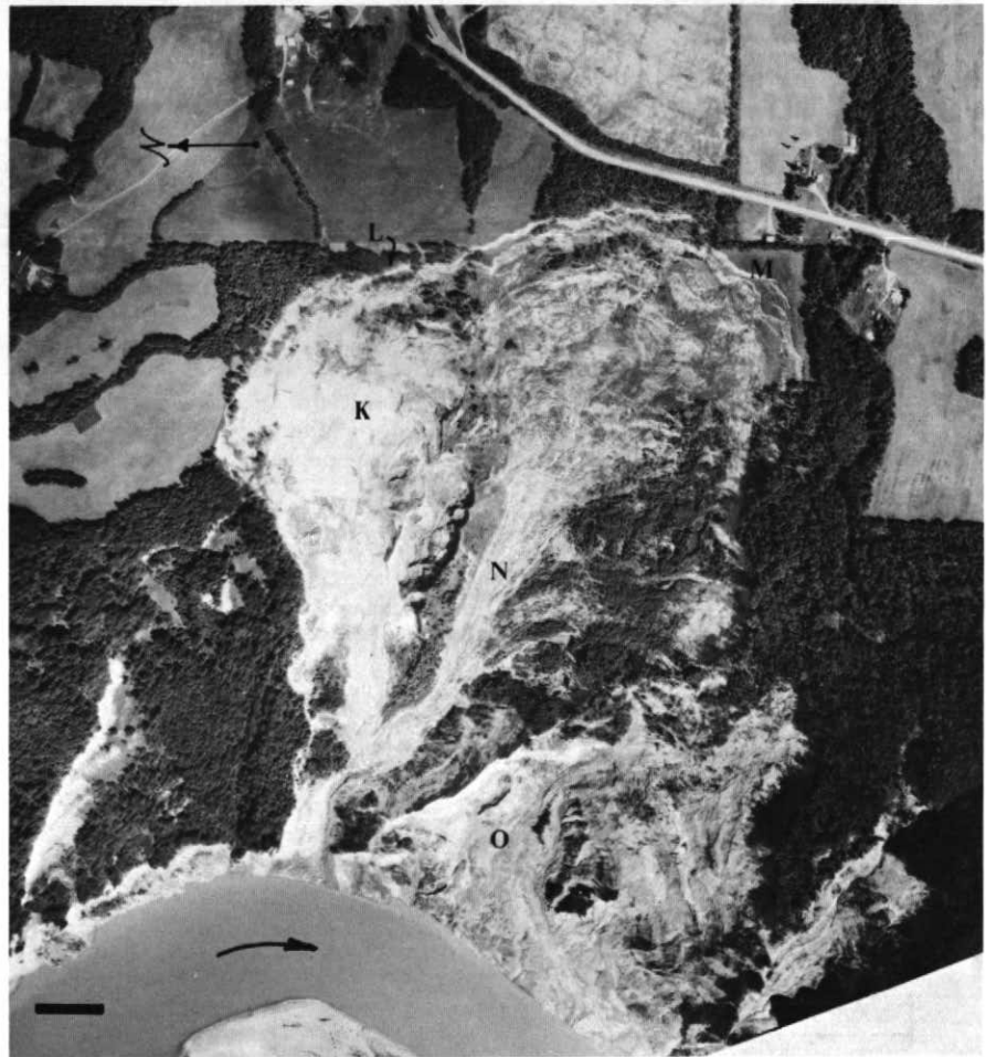
Figure 3: 1981 Air Photograph. K = North Bowl re-activated completely. Note broken ground. L = Active retrogression at North Bowl headscarp into in-situ glacio-lacustrine clay. M = Active retrogression at South Bowl headscarp has almost eliminated field (F in Fig. 2A). N =
