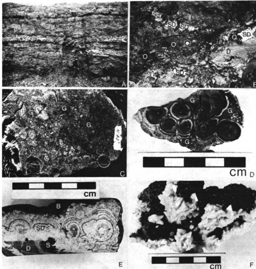
Figure 4 All views from Pine Point property, N.W.T. (A) - sagged solution breccia in Presqu'île dolomite (facies K; Skall, 1975), orebody N-38A; note abundant white sparry dolomite. (B) - close view of breccia in main ore zone, orebody N-38A; D, host dolomite; SD, white sparry dolomite; O, high-grade banded and colloform lead-zinc ore; 25¢ piece (circled) gives scale. (C) - high-grade ore showing colloform sphaerite (light to medium grey), infilled with massive galena (G, dark grey), orebody N-42;
