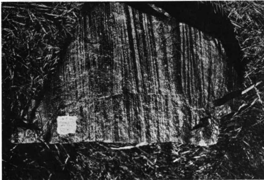
Figure 4 Banded stanniferous pyrrhotite exhalite ore from Luina Mine, northwest Tasmania. Photo by R. Ridler.
