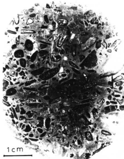
Figure 10 Iron formation deposited as muddy gravel. Intraclasts embedded in a micrite-type matrix. This is a storm layer deposited on top of a mud bank in the foreshore of the shelf. Hematite and magnetite predominate.
