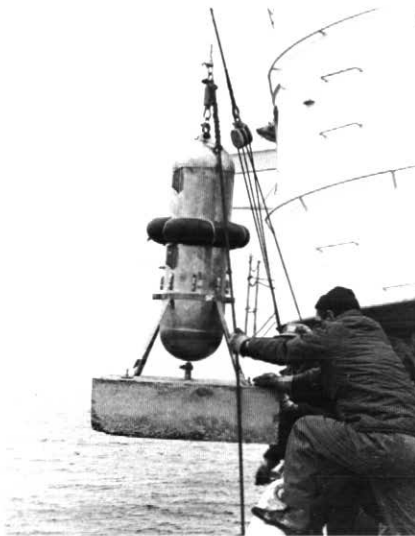
Figure 1 Offshore tide gauge developed by Tides and Water Levels, Marine Sciences Directorate, Department of the Environment. The inner tube senses pressure changes which are recorded internally on punched paper tape. (Bedford Institute of Oceanography).
