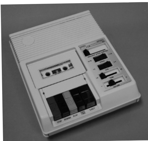
Figure 1. NLS C-1 "Cassette Book Machine." A bulky yellow plastic tape player, with large push buttons and slides for controlling volume, playback speed, rewind, and more. Courtesy of The Museum of the American Printing House for the Blind.
